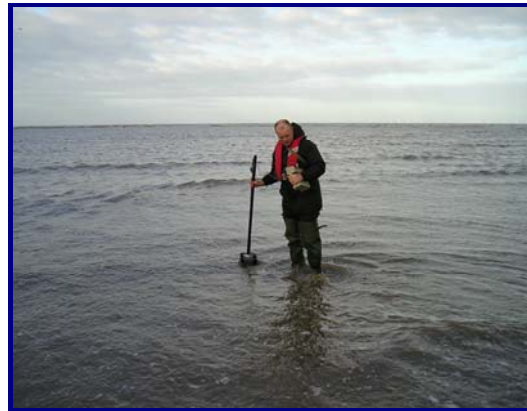
Measuring EMF over a buried cable.
